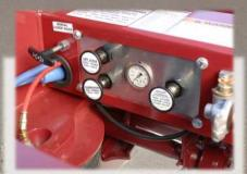
Adjustable Ride Height Control Adjustable ride height control is standard, with the controls conveniently located near the rear tail channel.
