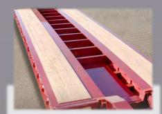
**Four-Beam Deck Design** The four-beam deck design can accommodate a wide range of loads, whether the weight is concentrated on the outside edges or in the middle of the trailer. The lightweight strength of Trail King's four-beam design also means you haul less trailer, more payload.
