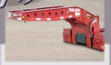
New Arched Gooseneck Design The new arched design provides ample truck frame clearance, even at the lowest king pin height setting. The gooseneck I-beam's web, top flange, and bottom flange feature one-piece construction for exceptional strength and durability. Externally mounted gooseneck stirrups are easy to service/replace.
